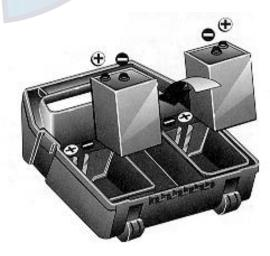
The Platinum ID Portable battery compartments have been designed to accept commercially available batteries with an overall height within industry tolerance. However, some batteries may be slightly shorter, preventing the spring terminals from contacting the brass terminal strips in the lower case. Should this occur, stretch the spring terminals slightly so that they contact the brass terminal strips in the lower case.
